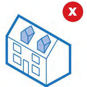
Loft conversion incorporating gable dormers which are out of scale and do not consider existing window rhythm or frequency.
